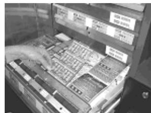
19. Multiple ticket packs can be loaded by taping the end of one pack to the beginning of another pack. To connect two packs, use GTECH's perforated tape (Part number 10-205-00007-01) and follow the instructions on the following page.
